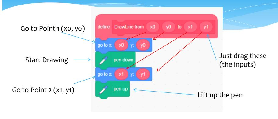
With this, we can draw a line starting from any (x0, y0) and ending at any (x1, y1) – We just need to provide these as inputs.
